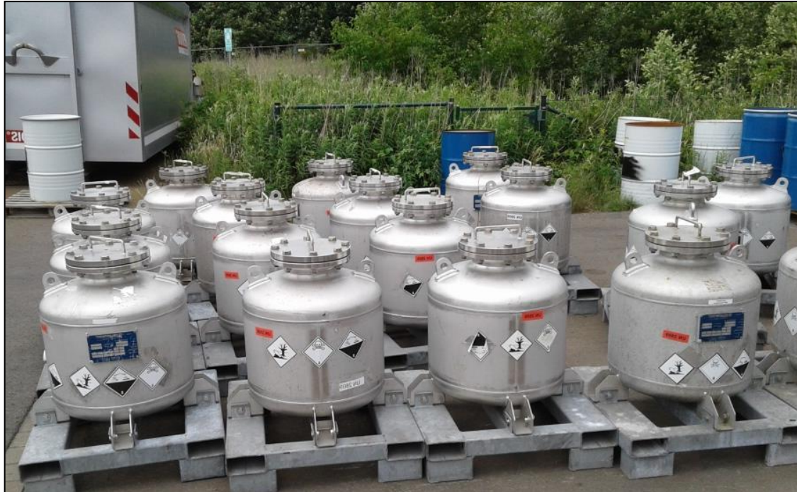
Example of metallic mercury container in preparation for road/sea transport (ADR, IMDG)
