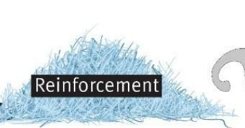
Reinforcement are used to reinforce or improve tensile strength, flexural strength and stiffness of the material. E.g. glass fibres, carbon fibres, etc.
